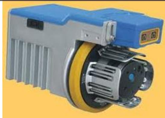
**Stopper:** It is an electronically controlled electromagnetic device integrated along with the accumulator. Its function in releasing the yarn at starts of insertion and stop it at the end of insertion.
