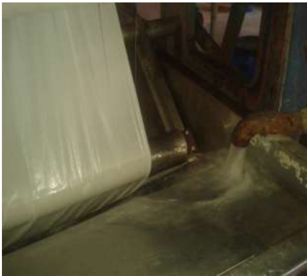
Filling of water in jigger machine
