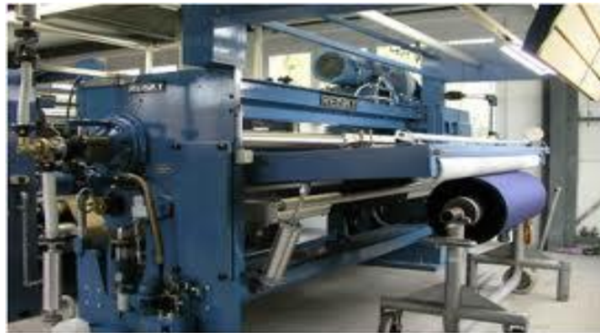
Out let batching device
