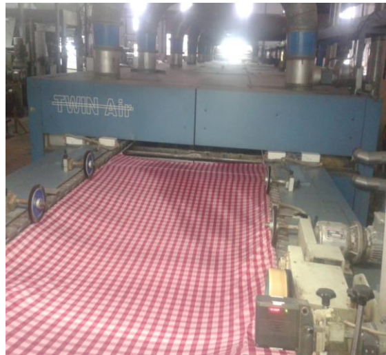
Proper feeding of fabric in chain track
