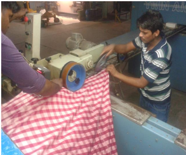
Proper feeding of fabric in chain track
