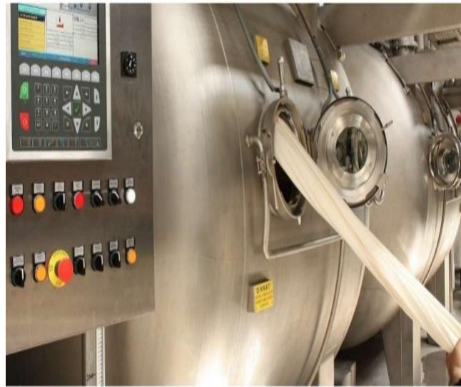
Loading of the machine inside main vessel
