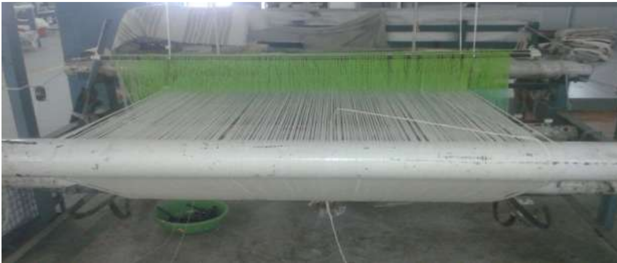
Broken Warp Ends
